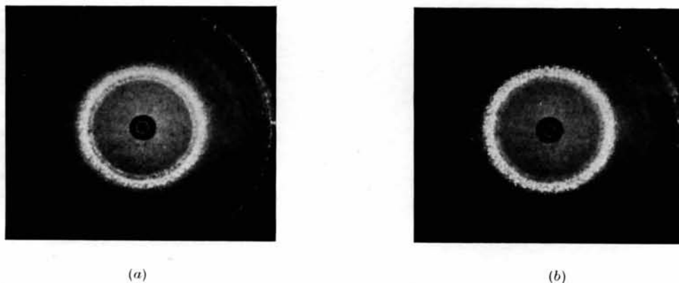
Fig. 1. Effect of electric field of 50 \text{ kV.cm.}^{-1} at 25^\circ \text{ C.} upon X-ray scattering in 4 \text{ BaTiO}_3 + 1 \text{ SrTiO}_3 . (a) Without field, (b) with field.
